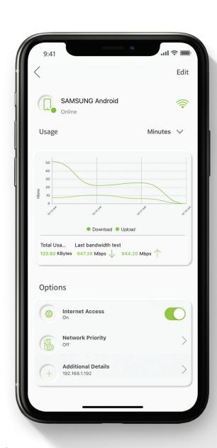
The Device details screen will show the device name at the top of the screen followed by a chart that indicates the amount of data that was used by the device over a period of time.
